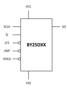
Figure 2. Pin Configuration SOP8 150/208 mil, TSSOP 173mil
