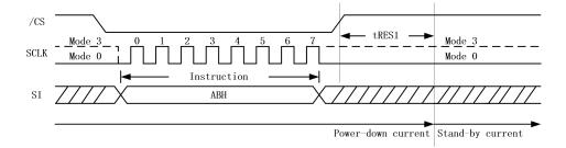
Figure 7.3.2b. Release Power-down / Device ID Instruction
