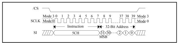
Figure 150. 32KB Block Erase with 4-Byte Address (QPI Mode)
