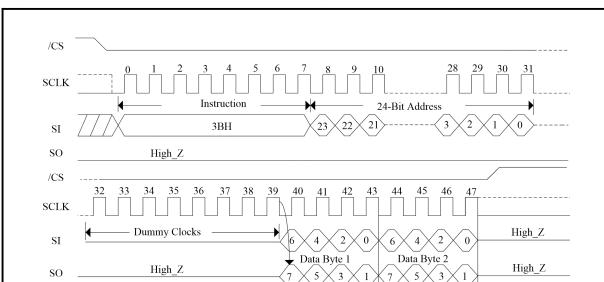
Figure 47. Dual Output Fast Read Sequence Diagram (SPI Mode/3-Byte Address Mode)
