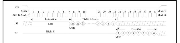
Figure 172. Read SPB Status (SPI Mode/4-Byte Address Mode)
