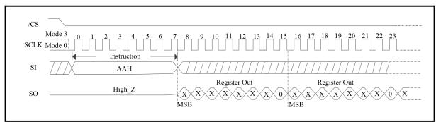
Figure 193. Read Unprotect Solid Protect Bit (SPI Mode)
