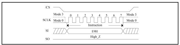
Figure 30. Exit 4-Byte Address Mode (QPI Mode)
