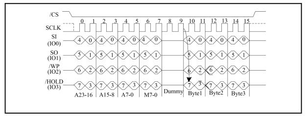
Figure 90. Quad I/O Word Fast Read Sequence Diagram (SPI Mode/4-Byte Address Mode; Initial instruction or previous (M5-4)=(1,0))
