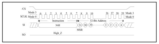
Figure 187. Dynamic Protection Block/Sector Lock (QPI Mode/3-Byte Address Mode)
