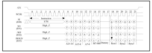
Figure 88. Quad I/O Word Fast Read Sequence Diagram (SPI Mode/4-Byte Address Mode; Initial instruction or previous (M5-4) $\neq$ (1,0))
