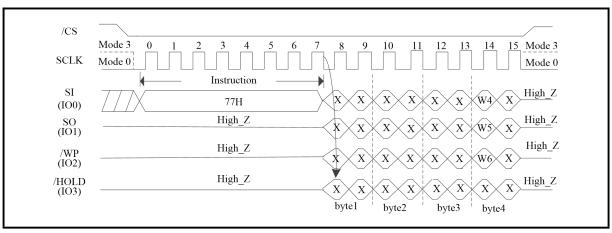
Figure 92. Set Burst with Wrap Sequence Diagram (SPI Mode only/4-Byte Address Mode)
