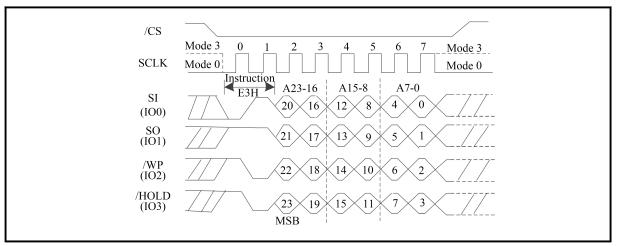
Figure 178. SPB Program (QPI Mode/4-Byte Address Mode)
