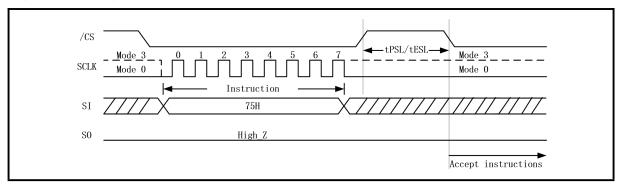
Figure 160. Program/Erase Suspend Instruction Sequence (QPI Mode)
