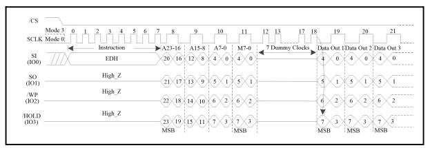
Figure 72. DTR Fast Read Quad I/O (SPI Mode/4-Byte Address Mode; Initial instruction or previous (M5-4 $\neq$ (1,0)))
