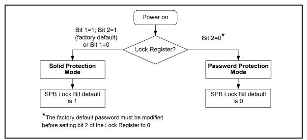
Figure 9. Enter Password Protection Mode
