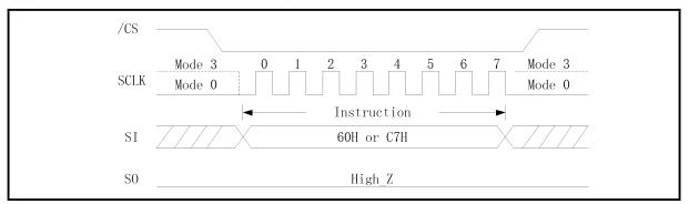
Figure 157. Chip Erase Sequence Diagram (SPI Mode)
