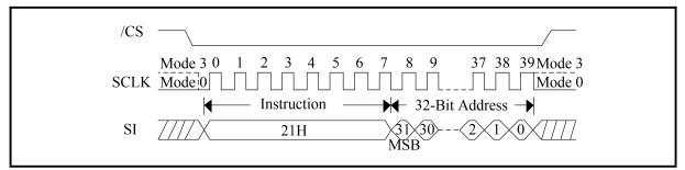
Figure 144. Sector Erase with 4-Byte Address (QPI Mode)
