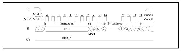
Figure 175. SPB Program (SPI Mode/3-Byte Address Mode)
