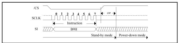
Figure 110. Deep Power-Down Sequence Diagram (SPI Mode)
