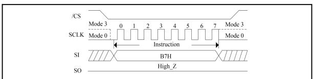
Figure 28. Enter 4-Byte Address Mode instruction (QPI Mode)
