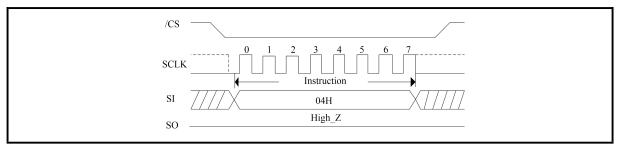
Figure 16. Write Disable Sequence Diagram (QPI Mode)
