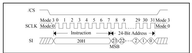
Figure 139. Sector Erase Sequence Diagram (SPI Mode/3-Byte Address Mode)
