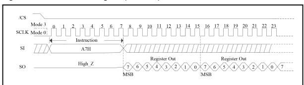
Figure 169. Read SPB Lock Register (SPI Mode)
