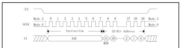
Figure 122. Erase Security Registers instruction Sequence Diagram (QPI Mode/3-Byte Address Mode)
