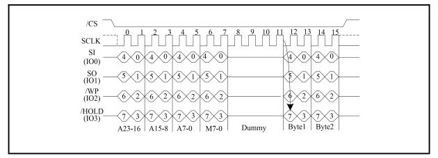
Figure 70. Quad I/O Fast Read Sequence Diagram (QPI Mode/4-Byte Address Mode; Initial instruction or previous (M5-4=(1,0)))
