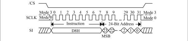
Figure 152. 64KB Block Erase Sequence Diagram (SPI Mode/4-Byte Address Mode)
