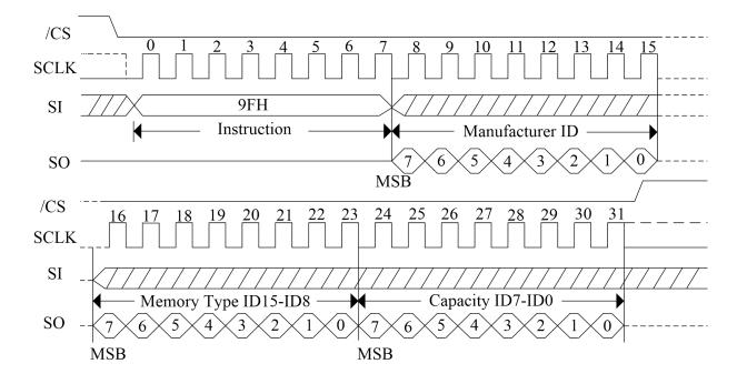
Figure 24. JEDEC ID Sequence Diagram
