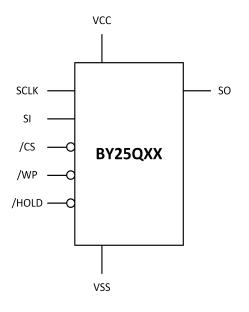
Figure 2. Pin Configuration SOP8
