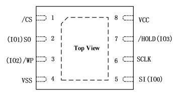
Figure 3.2. Pin Configuration DFN 4X3mm
