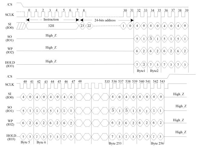
Figure 35.Quad Page Program Sequence Diagram
