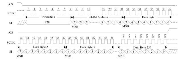
Figure 36.Fast Page Program Sequence Diagram
