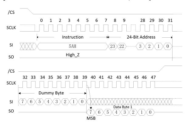
Figure 33. Read Serial Flash Discoverable Parameter command Sequence Diagram
