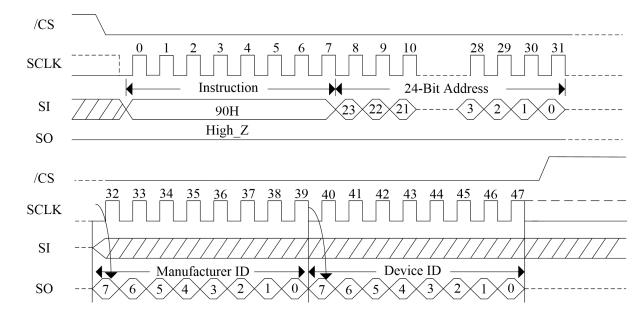
Figure 21. Read Manufacture ID/ Device ID Sequence Diagram
