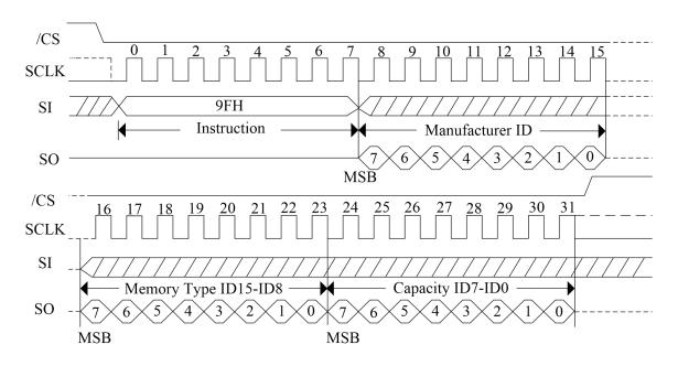
Figure 23.a. JEDEC ID Sequence Diagram (SPI Mode)
