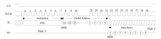
Figure 10. Read Data Bytes Sequence Diagram (SPI Mode only)
