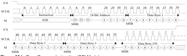
Figure 32.a. Page Program Sequence Diagram (SPI mode)
