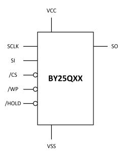
Figure 2. Pin Configuration SOP8
