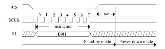
Figure 25.a. Deep Power-Down Sequence Diagram (SPI mode)
