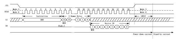
Figure 26.d. Release Power-down / Device ID Instruction (QPI Mode)
