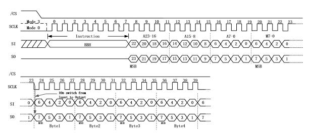
Figure 7.2.5a. Fast Read Dual I/O Instruction (Initial instruction or previous  $M5-4 \neq 10$ )
