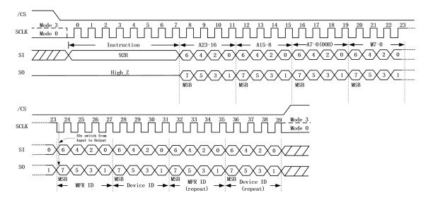
Figure 7.3.4. Read Manufacturer / Device ID Dual I/O Instruction
