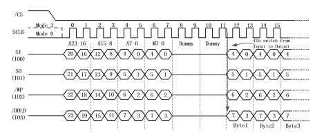
**Figure 7.2.6b.** Fast Read Quad I/O Instruction (Previous instruction set M5-4 = 10)
