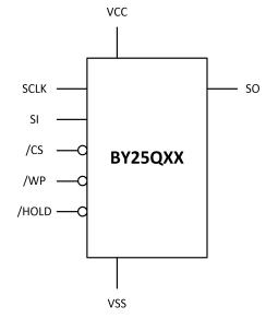
Figure 2. Pin Configuration SOP8/TSSOP8
