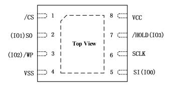
Figure 3.2. Pin Configuration USON8 4X3mm
