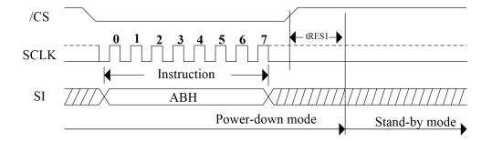
Figure 28. Release Power-Down/Read Device ID Sequence Diagram
