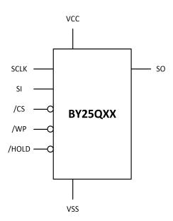
Figure 2. Pin Configuration SOP8
