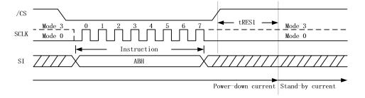
Figure 7.3.2b. Release Power-down / Device ID Instruction
