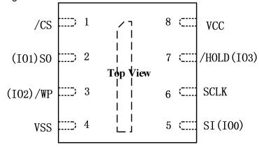
Figure 3.b. Pin Configuration DFN 1.5\*1.5mm
